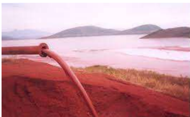
Fig 1. Discharge of Red Mud as Slurry into the Pond
